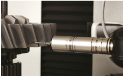
Tactile probing, for the complete inspection of a wide range of gear types, gear cutting tools and even non-gear, CMM-type measurement.
