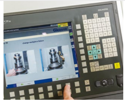
Menu-guided setup takes the operator through all the steps in the re-tooling process using helpful images.
