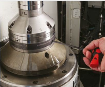
A single setup tool is all the operator needs to change over workholding, grippers and tools, helping to cut new part changeover time from 30-40 minutes to about 20 minutes.
