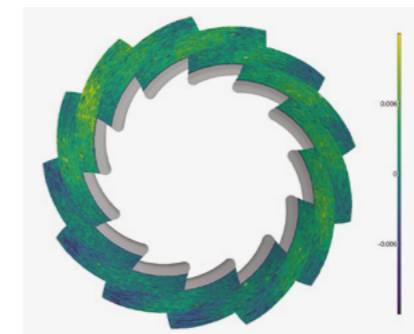
3D laser scan for cylindrical and bevel gears. Significant benefit for the reverse engineering of gears. Colors show variations from nominal data depending on the defined tolerance band.
