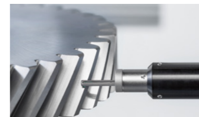
Non-skidded style probe provides surface roughness measurement capability as part of the normal gear inspection process, for gears down to module 1.5.
