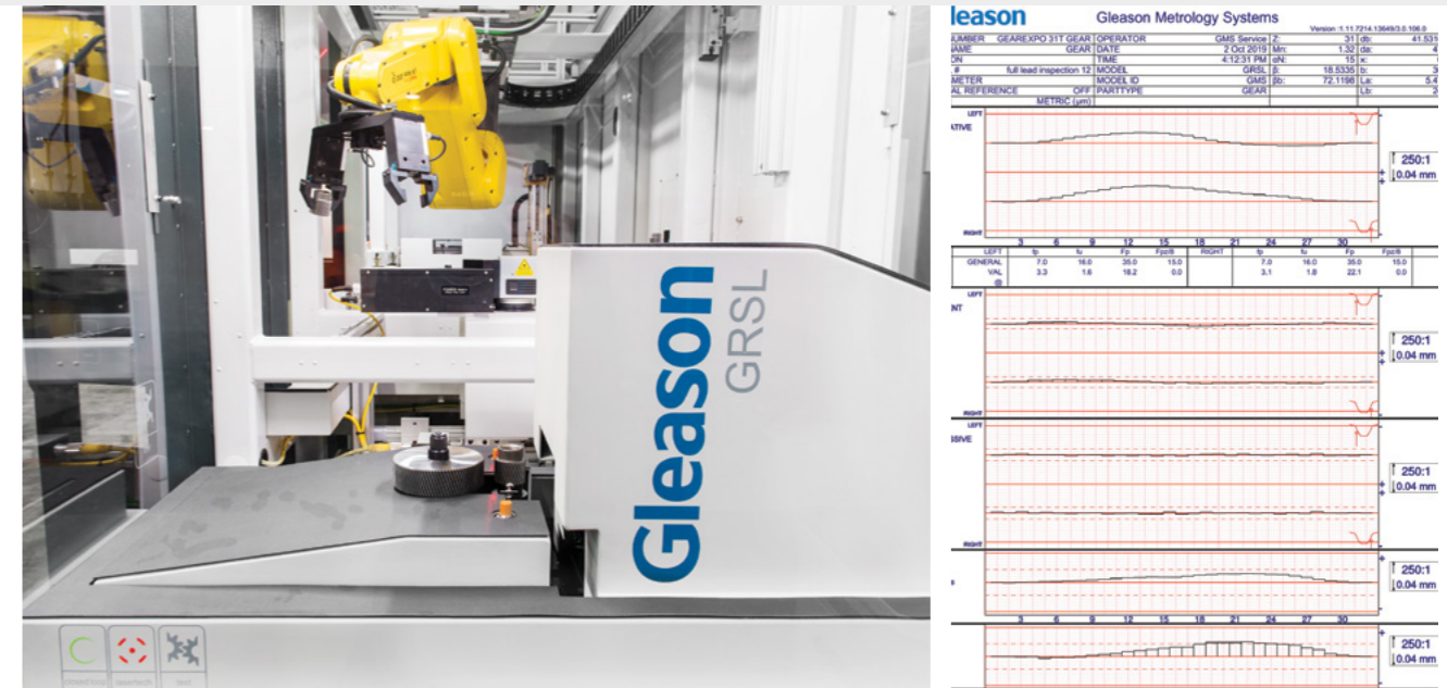
GRSL laser scanning validates parts in seconds, up to 100% of the entire output, with realtime feedback and advanced analytics including profile, lead and pitch measurement, as well as gear noise analysis.
