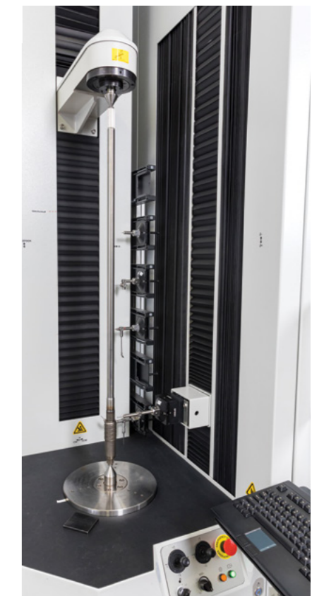
Shaft-type parts 1,000 mm in length can be accommodated. Tailstock with two speeds in both up and down directions and auto stop on achieved clamping force delivers faster, more consistent part loading/clamping.
