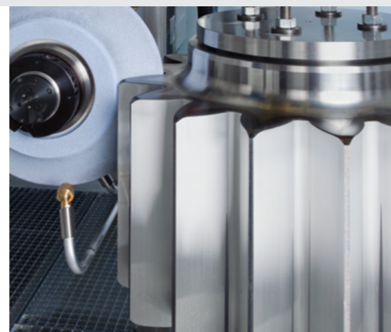
Grinding heads for external and internal gears accommodate dressable grinding wheels for maximum flexibility, CBN wheels for maximum stock removal.
