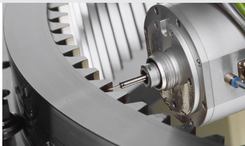
Integrated on-board inspection of internal and external gears to facilitate stock division, improving tool life and part quality.
