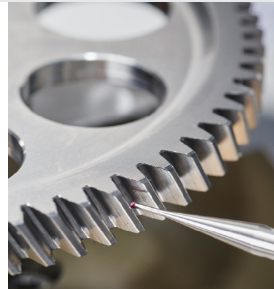
300GMS gives ODG the full range of inspection capabilities for a diverse range of projects, including noise analysis, fine pitch and even CMM-type measurement options.
