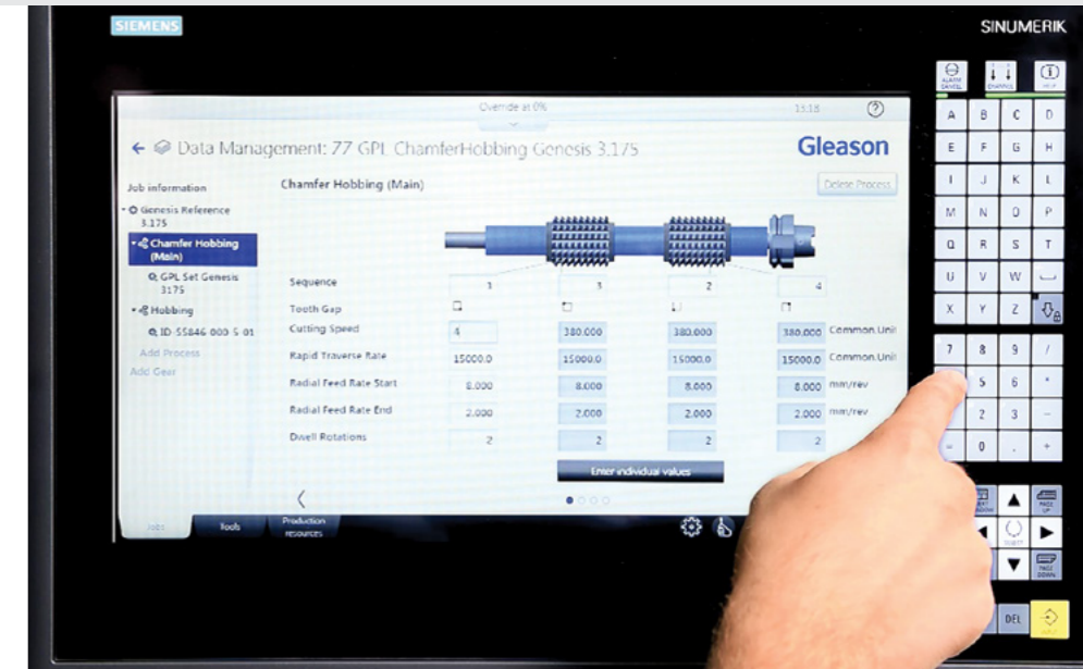
The newly developed GEMS® hobbing HMI allows intuitive and efficient operation of the entire hobbing-chamfering process chain.
