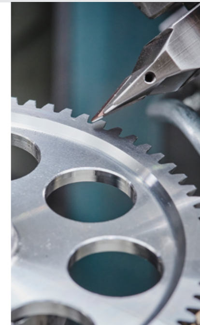
Fly Cutter Chamfering enables a relatively few different standard insert blade sets to accommodate a wide range of gear sizes, geometries and chamfer requirements.
