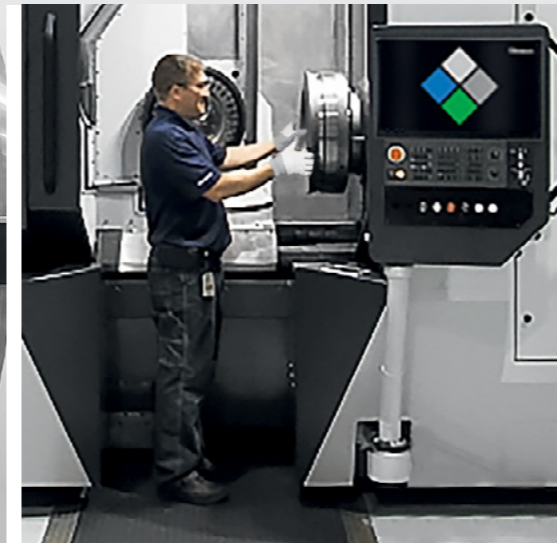
Operator works at floor level with no platform required to make cutter and workpiece changeover easier and faster.
