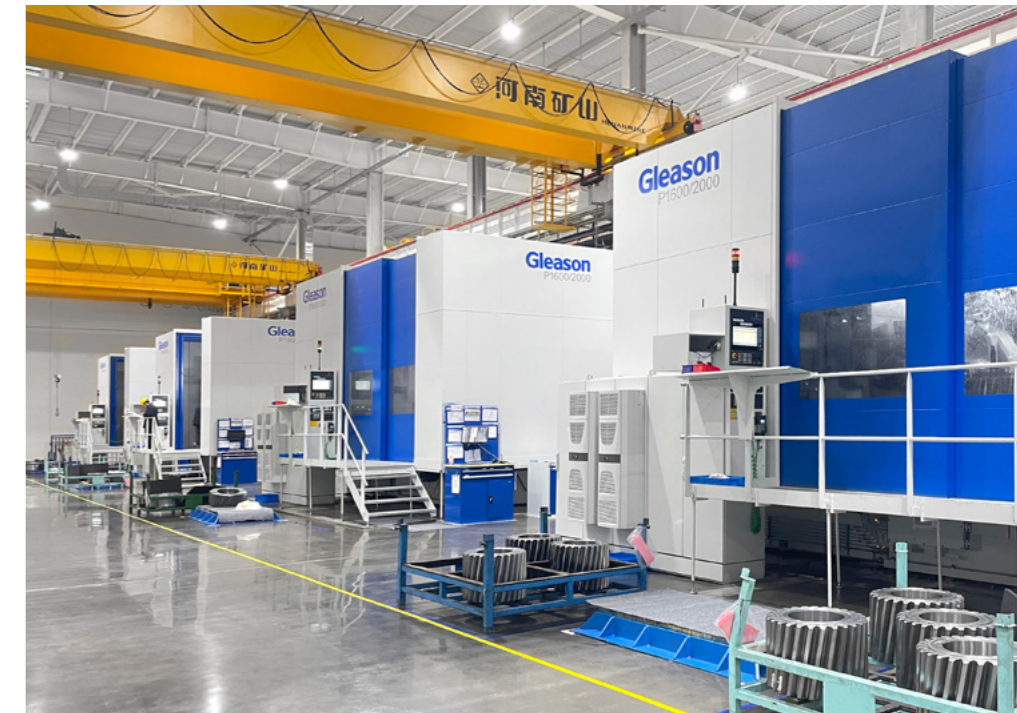
New P3200 Hobbing Machine adds much needed capacity for larger external and internal gears and shafts.
