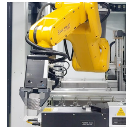
70ARC Automation System: Modular cart bay with robotic loading.
