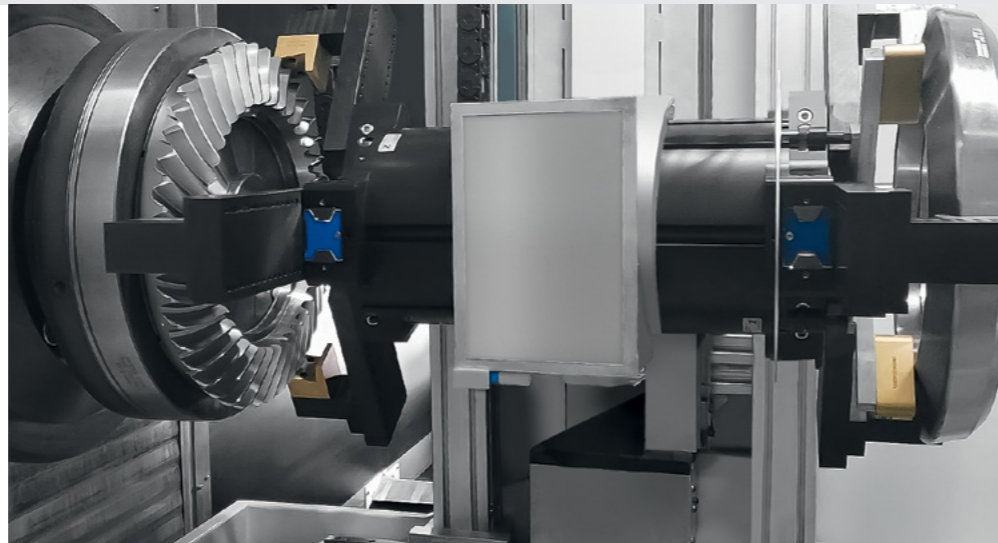
Robot loader automates the typically manual load/unload process of larger gear blanks and finish gears, cutting load/unload from minutes to as little as 22 seconds. The robot's dual grippers unload a finished part with one gripper, then swivel to load an uncut blank.
