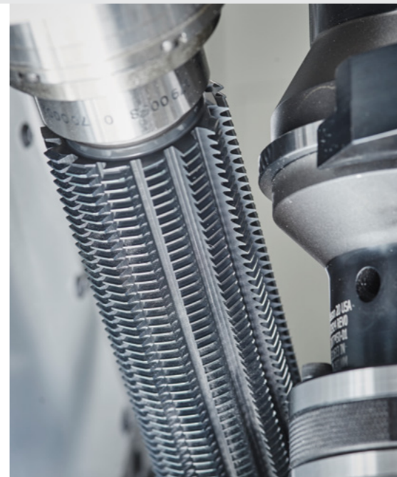
Hobbing and chamfering are done in parallel, thus eliminating significant non-productive time downstream.
