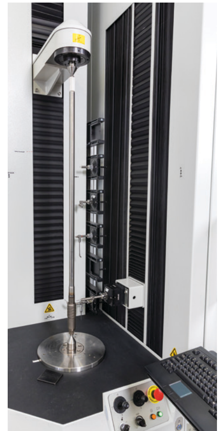
Shaft-type parts with 1,000 mm in length can be accommodated. Tailstock with two speeds in both up and down directions and auto stop on achieved clamping force delivers faster, more consistent part loading/clamping.
