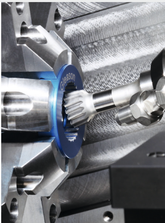
Power Skiving of internal gears.
