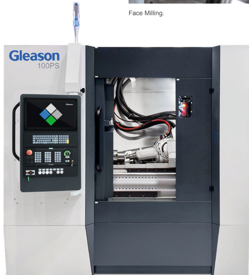
100PS Power Skiving machine features multiple processes on one platform.
